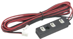
LED-CON3-350 Series power connector with (1) LED-END-350, 78" lead and mounting hole 2-1/4"L x 9/16"W
